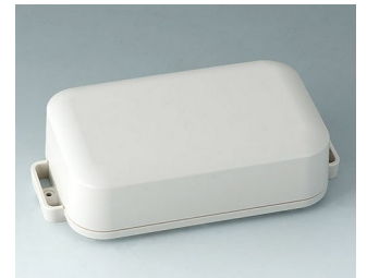
C3208207 EASYTEC 150 ASA+PC (UL 94 V-0) off-white RAL 9002 172x93x46mm IP 65 opt., IP 40
