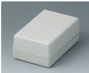
A9406341 SHELL-TYPE CASES G 110, Vers. I ABS (UL 94 HB) off-white RAL 9002 72x114x45mm IP 65 opt.
