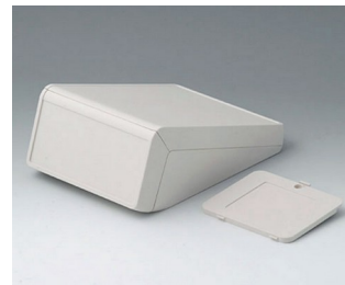
B4056327 UNITEC M, 1.4/0.6 ABS (UL 94 HB) off-white RAL 9002 148x210x80mm IP 40
