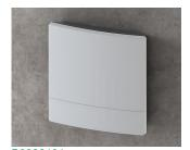
B3222101 NET-BOX 220, Vers. I ASA+PC (UL 94 V-0) light grey RAL 7035 220x220x50,5mm IP 65 opt., IP 40
