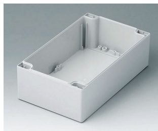
C2122002 Case shell 120, with tongue PC (UL 94 HB) light grey RAL 7035 200x120x60mm
