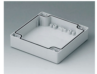
C1121202 Case shell 120, with groove PC (UL 94 HB) light grey RAL 7035 120x120x30mm
