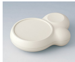
B2512107 BLOB CONTROL ABS (UL 94 HB) off-white RAL 9002 114x76x31mm IP 54 opt.
