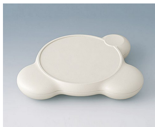
B2514107 BLOB PANEL ABS (UL 94 HB) off-white RAL 9002 200x165x36mm IP 54 opt.
