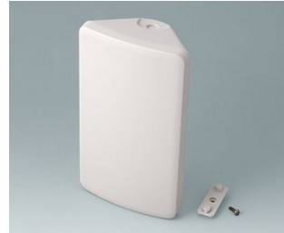
B4610107 SMART-CONTROL M, Vers. I ASA+PC (UL 94 V-0) off-white RAL 9002 173x101x59mm IP 55 opt., IP 40
