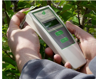
Chlorophyll fluorimeter for plant screening
