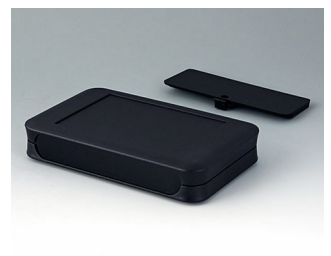
A9053219 SOFT-CASE XL PMMA (IR) (UL 94 HB) black RAL 9005 92x150x28mm IP 40
