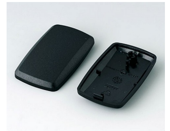
B9002856 Bottom and top part ES PMMA (IR) (UL 94 HB) black RAL 9005 52x32x15mm
