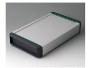
B3407031 SMART-TERMINAL 240 Aluminium AIMgSi 0,5 matt anodised 282x170x50mm IP 54
