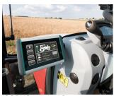
ISOBUS terminal for tractors and self-propelled machines
