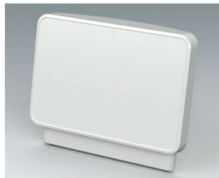
C3604407 Operating panel M ASA+PC (UL 94 V-0) traffic white RAL 9016 328x78x275mm
