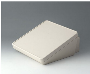
B4422307 PROTEC 220, Vers. III ASA+PC-FR (UL 94 V-0) off-white RAL 9002 220x243x108mm IP 65 opt.
