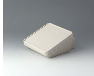
B4414307 PROTEC 140, Vers. III ASA+PC-FR (UL 94 V-0) off-white RAL 9002 140x160x76mm IP 65 opt.
