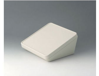
B4418107 PROTEC 180, Vers. I ASA+PC-FR (UL 94 V-0) off-white RAL 9002 180x180x92mm IP 65 opt.
