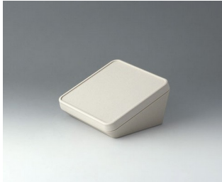
B4414107 PROTEC 140, Vers. I ASA+PC-FR (UL 94 V-0) off-white RAL 9002 140x140x76mm IP 65 opt.
