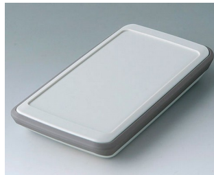
B5403317 SLIM-CASE M, Vers. VI ASA+PC-FR (UL 94 V-0) off-white RAL 9002 148x74x22mm IP 54
