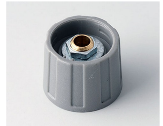
A2520068 ROUND KNOB 20, without line ABS (UL 94 HB) dusty grey RAL 7037 20x15mm 6mm
