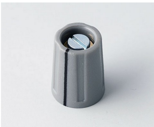
A2610038 ROUND KNOB 10, with line ABS (UL 94 HB) dusty grey RAL 7037 10x14mm 3mm
