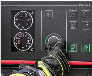
Control element for pump control station
