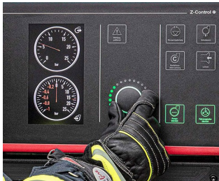
Control element for pump control station
