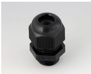
C2316419 Cable gland M16x1.5 PA 6 black RAL 9005 IP 68 opt.
