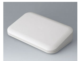
A9465107 EVOTEC 200, Vers. II ASA+PC-FR (UL 94 V-0) off-white RAL 9002 200x124x45mm IP 65 opt., IP 40
