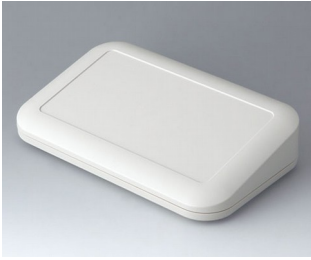
A9466107 EVOTEC 200, Vers. III ASA+PC-FR (UL 94 V-0) off-white RAL 9002 200x124x45mm IP 65 opt., IP 40
