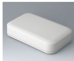
A9461107 EVOTEC 200, Vers. I ASA+PC-FR (UL 94 V-0) off-white RAL 9002 200x124x45mm IP 65 opt., IP 40
