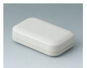
A9401107 EVOTEC 80, Vers. I ASA+PC (UL 94 V-0) off-white RAL 9002 80x50x22mm IP 65 opt., IP 40
