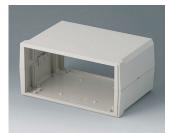
B3020137 MOTEC M, high/high ABS (UL 94 HB) off-white RAL 9002 205x140x100mm IP 40
