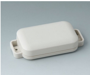
C3204107 EASYTEC 80 ASA+PC-FR (UL 94 V-0) off-white RAL 9002 101x50x22mm IP 65 opt., IP 40
