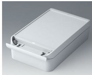
C6013221 SMART-BOX WIDTH 130 ASA+PC-FR (UL 94 V-0) light grey RAL 7035 220x130x60mm IP 66
