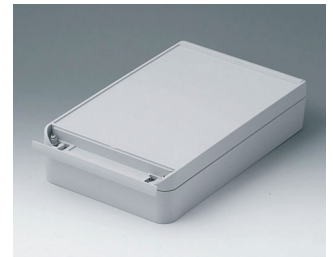
C6017281 SMART-BOX WIDTH 170 ASA+PC-FR (UL 94 V-0) light grey RAL 7035 280x170x60mm IP 65
