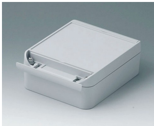
C6013161 SMART-BOX WIDTH 130 ASA+PC-FR (UL 94 V-0) light grey RAL 7035 160x130x60mm IP 66
