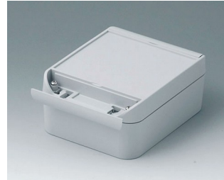
C6011141 SMART-BOX WIDTH 110 ASA+PC-FR (UL 94 V-0) light grey RAL 7035 140x110x60mm IP 66
