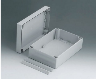
C2116241 ROBUST-BOX WIDTH 160, Vers. I ABS (UL 94 HB) light grey RAL 7035 240x160x90mm IP 66
