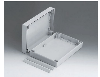
C2016242 ROBUST-BOX WIDTH 160, Vers. II PC (UL 94 HB) light grey RAL 7035 240x160x60mm IP 66
