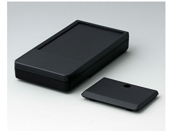
A9072219 DATEC-POCKET-BOX L ABS (UL 94 HB) black RAL 9005 120x65x22mm IP 54
