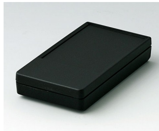
A9070219 DATEC-POCKET-BOX S PMMA (IR) (UL 94 HB) black RAL 9005 85x46x16mm IP 54
