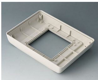
B4042767 Bottom part S high, version II ABS (UL 94 HB) off-white RAL 9002 190x135x34.5mm IP 54 opt.
