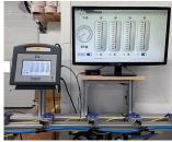
Monitoring system for cleaning nozzles
