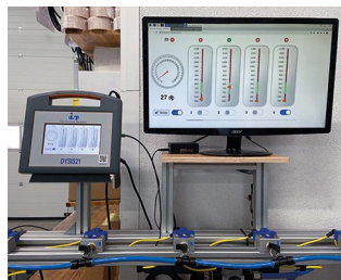
Monitoring system for cleaning nozzles
