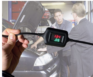
Voltage and current display during trickle charging
