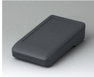
A9005108 DATEC-COMPACT S ASA+PC (UL 94 V-0) lava 136x74x32mm IP 65
