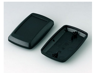
B9006816 Bottom and top part EL PMMA (IR) (UL 94 HB) black RAL 9005 78x48x24mm
