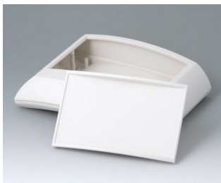
B7020237 ERGO-CASE L, flat ABS (UL 94 HB) off-white RAL 9002 150x200x54mm IP 40
