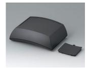
B7025109 ERGO-CASE L, high ABS (UL 94 HB) black RAL 9005 150x200x69mm IP 54 opt.
