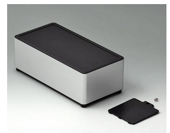
EE206059 SYNERGY E200 Aluminium AIMgSi 0.5 matt anodised 200x100x70mm IP 40
