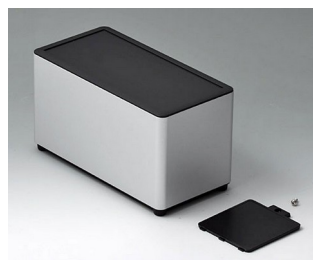
EE189059 SYNERGY E180 Aluminium AIMgSi 0.5 matt anodised 180x90x100mm IP 40
