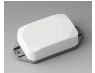
B1822226 MINI-DATA-BOX EF40, high, with flanges ASA+PC (UL 94 V-0) traffic white RAL 9016 60x40x20mm IP 65 opt., IP 40
