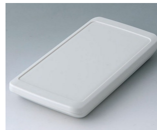
B5403207 SLIM-CASE M, Ausf. II ASA+PC (UL 94 V-0) grauweiß RAL 9002 148x74x19mm IP 65 opt., IP 40
