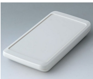
B5403307 SLIM-CASE M, Ausf. III ASA+PC (UL 94 V-0) grauweiß RAL 9002 148x74x19mm IP 65 opt., IP 40
