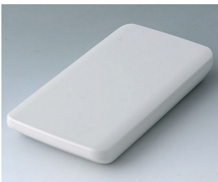
B5403107 SLIM-CASE M, Ausf. I ASA+PC (UL 94 V-0) grauweiß RAL 9002 148x74x19mm IP 65 opt., IP 40
