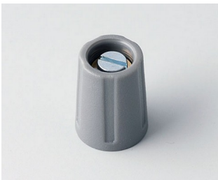
A2510038 RUNDKNOPF 10, ohne Strich ABS (UL 94 HB) staubgrau RAL 7037 10x14mm 3mm
