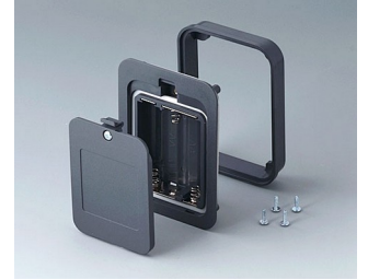
A9336118 Batteriefach-Set, 3 x AA ABS (UL 94 HB) lava 93x69mm IP 54
