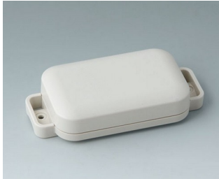
C3204107 EASYTEC 80 ASA+PC (UL 94 V-0) grauweiß RAL 9002 101x50x22mm IP 65 opt., IP 40
