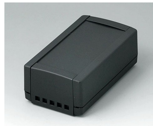
B1050469 TOPTEC 123 H, Ausf. II ABS (UL 94 HB) schwarz RAL 9005 123x68x45mm IP 40
