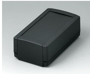
B1050369 TOPTEC 123 H, Ausf. I ABS (UL 94 HB) schwarz RAL 9005 123x68x45mm IP 40
