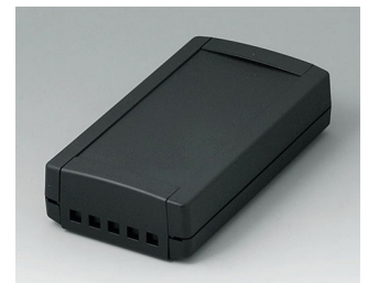
B1065469 TOPTEC 154 F, Ausf. II ABS (UL 94 HB) schwarz RAL 9005 154x84x38mm IP 40
