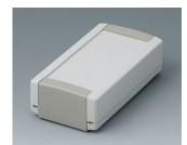
B1040365 TOPTEC 102, Ausf. I ABS (UL 94 HB) grauweiß RAL 9002 102x54x30mm IP 40
