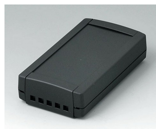
B1055469 TOPTEC 123 F, Ausf. II ABS (UL 94 HB) schwarz RAL 9005 123x68x30mm IP 40
