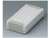
B1065365 TOPTEC 154 F, Ausf. I ABS (UL 94 HB) grauweiß RAL 9002 154x84x38mm IP 40
