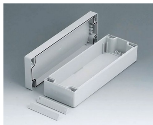
C2008242 ROBUST-BOX 80 BREIT, Ausf. II PC (UL 94 HB) lichtgrau RAL 7035 240x80x60mm IP 66
