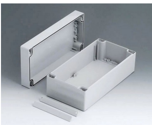
C2112241 ROBUST-BOX 120 BREIT, Ausf. I ABS (UL 94 HB) lichtgrau RAL 7035 240x120x90mm IP 66
