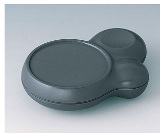
B2512108 BLOB CONTROL ABS (UL 94 HB) lava 114x76x31mm IP 54 opt.
