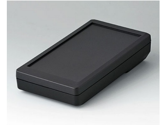
A9073119 DATEC-MOBIL-BOX S, Ausf. I ABS (UL 94 HB) schwarz RAL 9005 152x83x33,5mm IP 65 opt.
