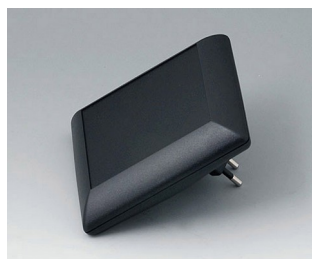
B5013229 ART-CASE S110 F PC+ABS (UL 94 V-0) schwarz RAL 9005 110x110x38mm IP 40
