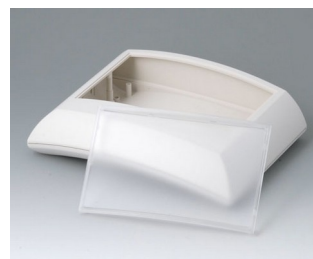
B7020247 ERGO-CASE L, flach ABS (UL 94 HB) grauweiß RAL 9002 150x200x54mm IP 40
