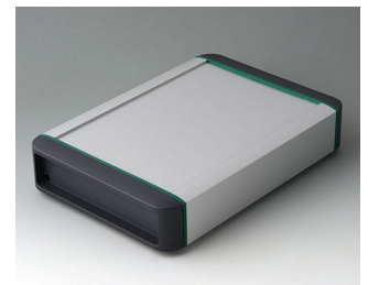
B3407021 SMART-TERMINAL 200 Aluminium AlMgSi 0,5 matt eloxiert 242x170x50mm IP 54
