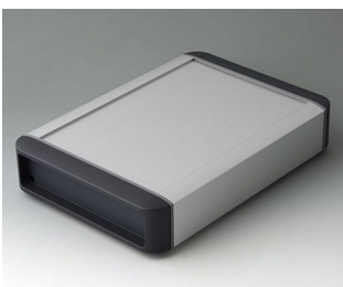
B3407022 SMART-TERMINAL 200 Aluminium AlMgSi 0,5 matt eloxiert 242x170x50mm IP 54
