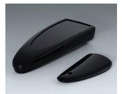
B2804016 STYLE-CASE L PMMA (IR) (UL 94 HB) schwarz RAL 9005 166x64x31mm IP 65 opt., IP 40
