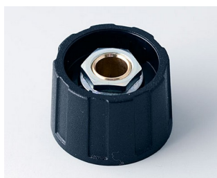
A2523060 ROUND KNOB 23, without line ABS (UL 94 HB) black RAL 9005 23x15mm 6mm
