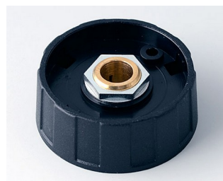
A2540080 ROUND KNOB 40, without line ABS (UL 94 HB) black RAL 9005 40x15mm 8mm
