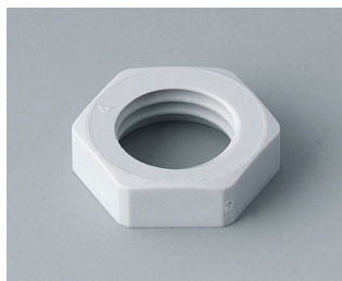
C2312117 Counternut M12x1.5 PA 6 light grey RAL 7035
