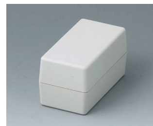
A9404441 SHELL-TYPE CASES G 85, Vers. I ABS (UL 94 HB) off-white RAL 9002 45x85x45mm IP 65 opt.
