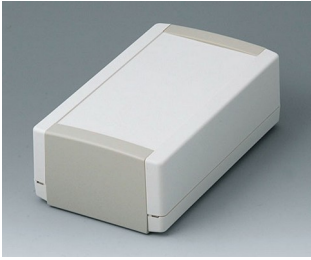
B1070365 TOPTec 194 H, Vers. I ABS (UL 94 HB) off-white RAL 9002 194x115x68mm IP 40
