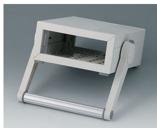
B2213117 MEDITEC E 160, with handle bar ABS (UL 94 HB) off-white RAL 9002 160x200x74mm IP 40
