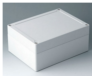
C7021071 IN-BOX ABS (UL 94 HB) light grey RAL 7035 202x152x90mm IP 66, IP 67, IK 07
