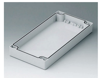
C1122402 Case shell 120, with groove PC (UL 94 HB) light grey RAL 7035 240x120x30mm
