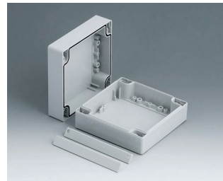
C2012121 ROBUST-BOX WIDTH 120, Vers. I ABS (UL 94 HB) light grey RAL 7035 120x120x60mm IP 66
