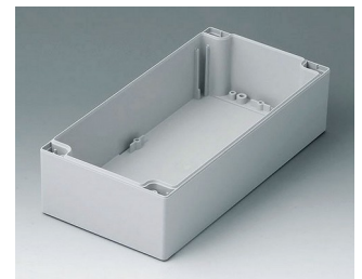
C2122401 Case shell 120, with tongue ABS (UL 94 HB) light grey RAL 7035 240x120x60mm
