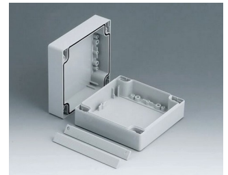
C2012122 ROBUST-BOX WIDTH 120, Vers. II PC (UL 94 HB) light grey RAL 7035 120x120x60mm IP 66
