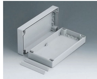
C2012241 ROBUST-BOX WIDTH 120, Vers. I ABS (UL 94 HB) light grey RAL 7035 240x120x60mm IP 66
