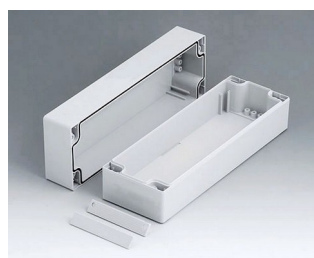
C2108241 ROBUST-BOX WIDTH 80, Vers. I ABS (UL 94 HB) light grey RAL 7035 240x80x80mm IP 66
