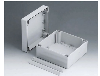
C2116162 ROBUST-BOX WIDTH 160, Vers. II PC (UL 94 HB) light grey RAL 7035 160x160x90mm IP 66
