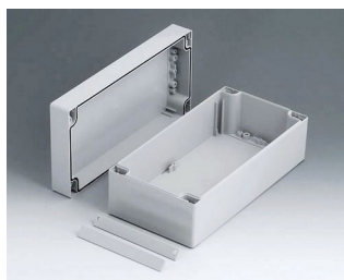
C2112241 ROBUST-BOX WIDTH 120, Vers. I ABS (UL 94 HB) light grey RAL 7035 240x120x90mm IP 66
